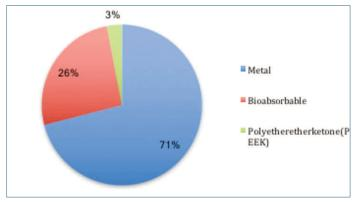
Figure 21: Materials used for tibial tunnel interference screws
